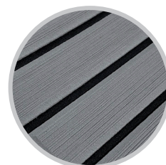
Competitor Sample Foam discolouration after 500 hours
