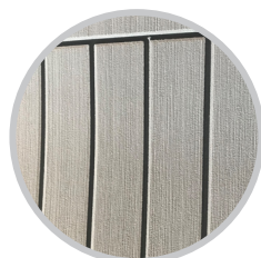
Competitor Sample Foam discolouration after 500 hours
